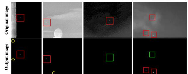
Fig. 18. Output results of PGDN-Net2. The red box indicates that the real target is detected, the green box indicates that the real target is lost, and the yellow circle marks the clutter and false target points present in the background.
