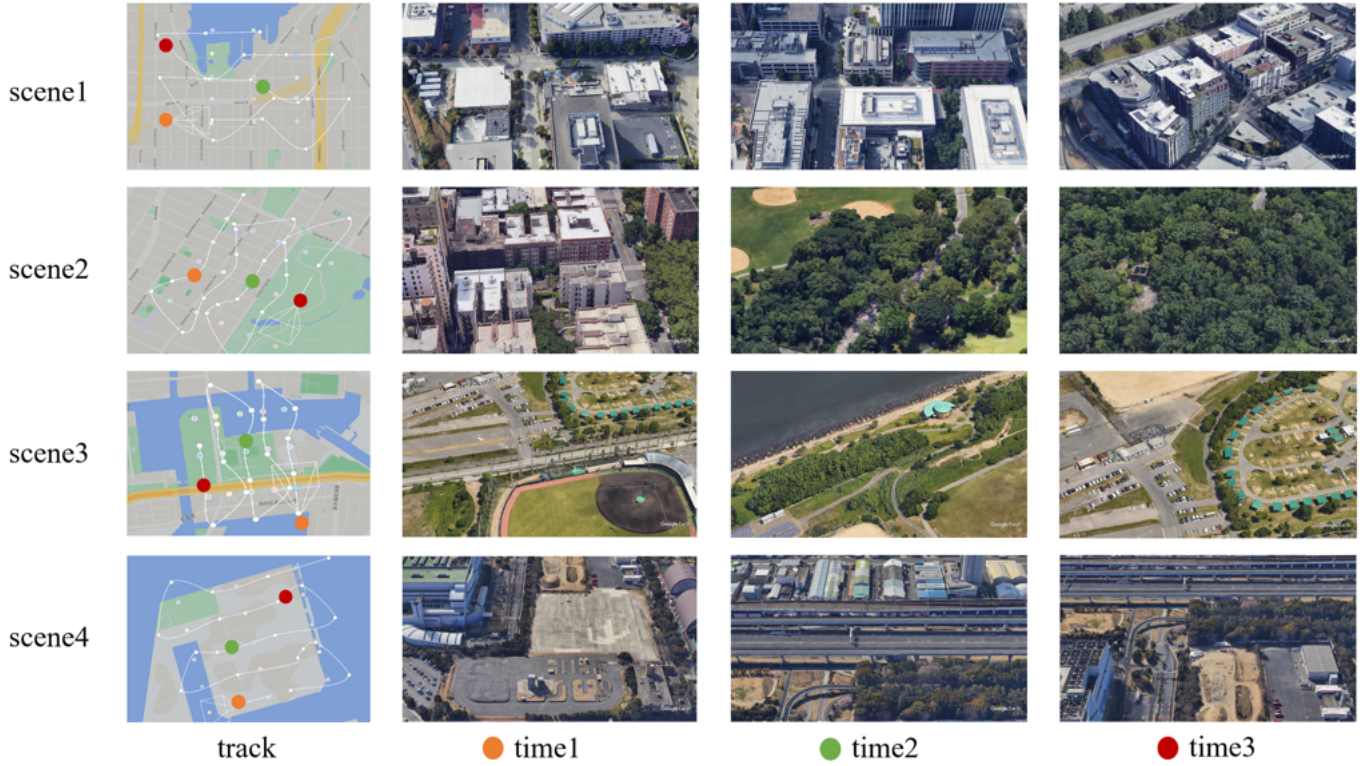
Fig. 7: Trajectories of the first four scenes and forward-looking images at different times. The leftmost images show the camera trajectories (white curves) from a forward-looking perspective for four scenes. White dots indicate the key points selected during the trajectory design, with camera poses for the remaining frames obtained using cubic spline interpolation for a smooth trajectory. The orange, green, and red dots represent the camera’s position at three specific moments, corresponding to the images shown in the right three columns.
