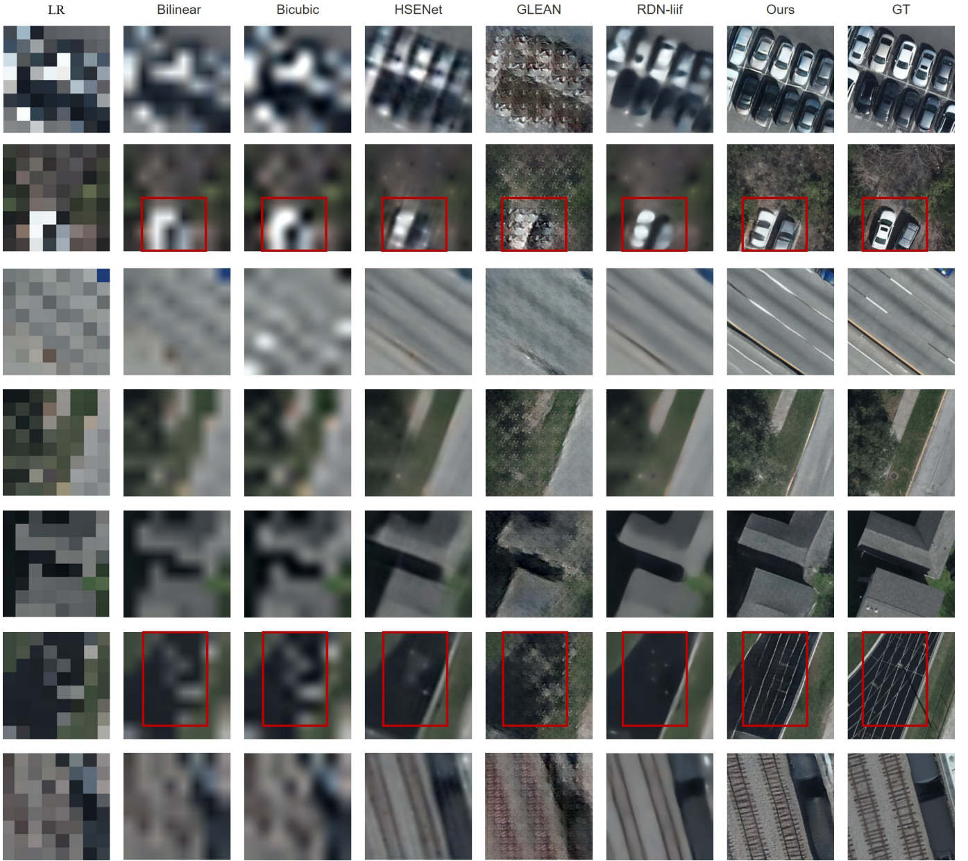
Fig. 6. Visual comparison of different methods. From 1st to 8th column: low resolution input (32x), bilinear interpolation, bicubic interpolation, HSENet [21], GLEAN [20], RDN-liif [29], our result, and ground truth. It can be seen that for lawns, roofs, playgrounds, parking lots, roads, rails, and other types of ground objects, our output results are superior to similar networks in terms of semantic accuracy, edge, texture, and other details. For small-scale targets that are mixed in a single-pixel grid, our super-resolution idea can effectively realize sub-pixel level unmixing, and clearly define the meaning and geographical location of objects. On this basis, our network can effectively generate image texture with the help of rich and diverse priors. For example, the unique texture of the parking lot line, playground runway line, roof, and lawn texture.
