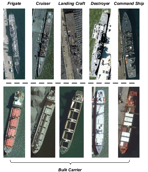
Fig. 1. The challenge of high inter-class similarity and low intra-class similarity in FGSC task in RS. In the first row, ships of different subclasses are similar in appearance, while in the second row, ship appearances of the same subclass are quite different.
