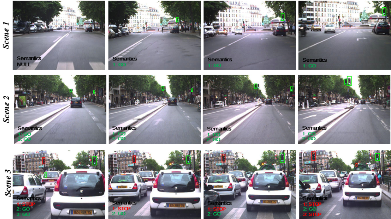
Fig. 14. Traffic light detection results on TLR dataset [15]. In scene 2, a green light is missed. In scene 3, a false detection is made since a spot reflected by the mirror resembles a green traffic light both in color and shape. These false results cannot be easily excluded, unless it is used in correlation to other computer vision modules like a vehicle detector or a road detector [23].
