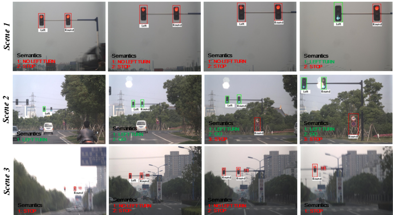
Fig. 9. Some traffic detection results of our system. In scene 2, a traffic sign is falsely detected as a red light, and a green light is missed since the target is too far. In scene 3, a red light is missed since the frames are blurred by the motion of the vehicle. Due to the limited space, each frame is cropped to 750 \times 1000 pixels for illustration.
