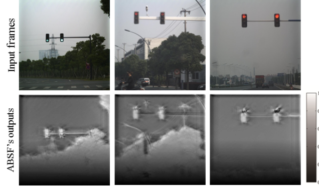
Fig. 4. AdaBSF's results of frame captured under different light conditions. The first row shows the original input frames. The second row shows the AdaBSF's filtering results. Noticed that traffic lights usually appears in the upper half part of the scene, we have manually reduced the score at the very bottom of each output map.
