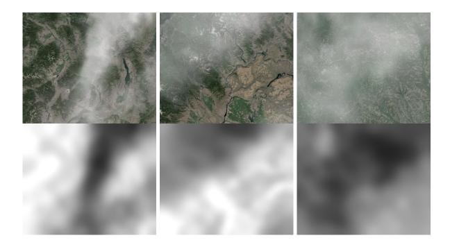
Fig. 4. Instances of extracted transmissions, where the first row shows hazy images and the second row shows their corresponding transmissions.
