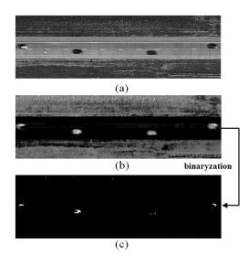
**Fig. 4**. Example for application in car detection. (a) The original image. (b) One abundance map. (c) The abundance map with image thresholding.
