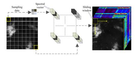
Fig. 2. Illustration of HSI simulating process with PI.
