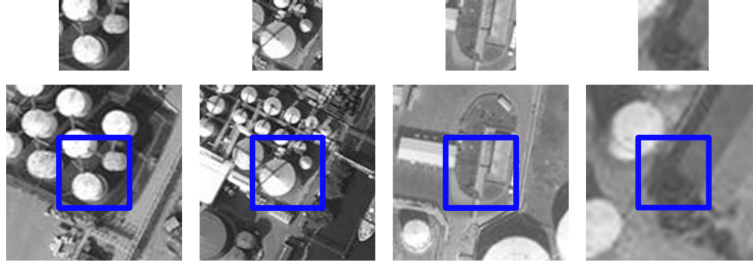
Fig. 4. Some negative samples whose surrounding areas include some oil tanks. These samples announced by the modified ELSD are cut from different images. The first row indicates the local patches, the second row refers to their corresponding surroundings. The positions of the local patches are shown with rectangles in their corresponding surrounding areas.
