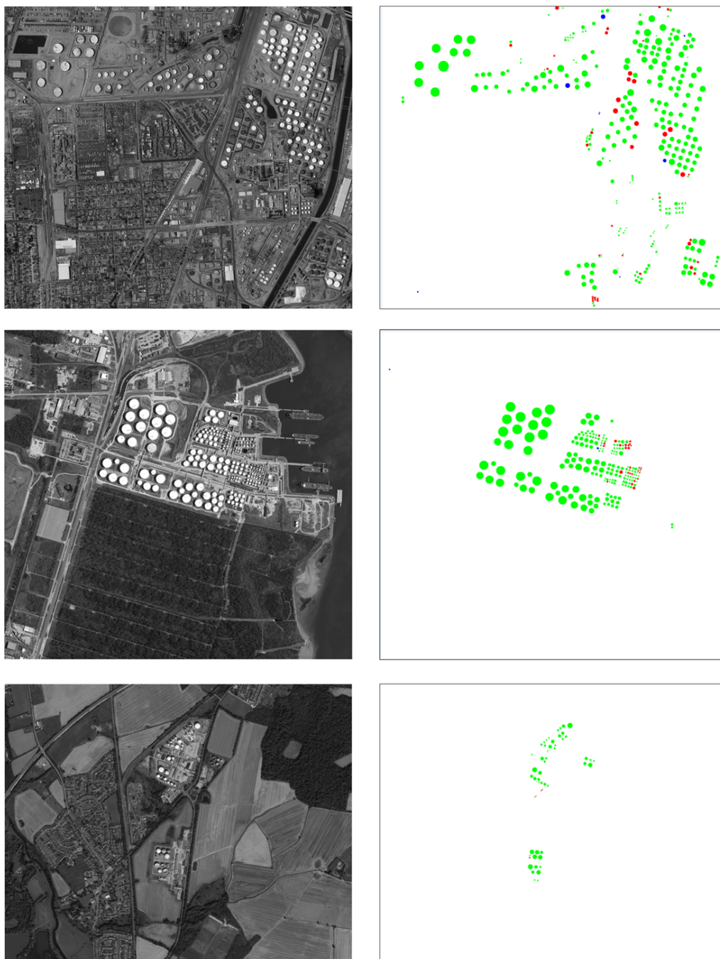
Fig. 17. Detection results with LHO-SCNN feature in the large size images. The size of the image in the first row is 2781 \times 2445 , the longitude is -118.238100 and the latitude is 33.801487 . The size of the image in the second row is 2158 \times 2290 , the longitude is -95.128800 and the latitude is 29.744275 . The size of the image in the third row is 3712 \times 3008 , the longitude is -1.672366 and the latitude is 52.571756 .
