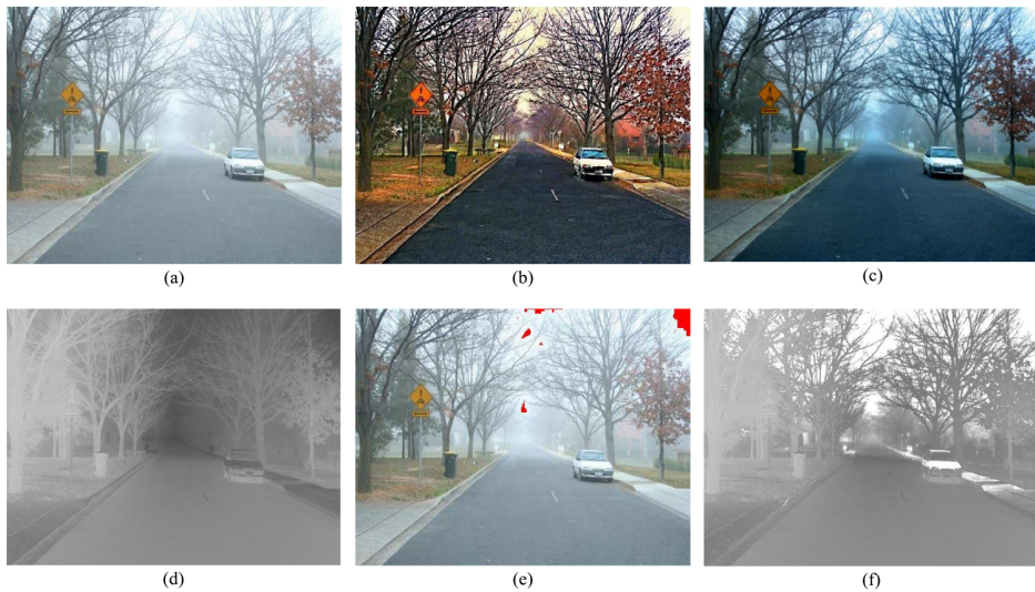
Fig. 5: Comparison with Tan’s work [7]. (a) Input hazy image. (b) Tan’s result. (c) Our result. (d) Refined transmission. (e) Detected sky region. (f) Our adjusted transmission.
