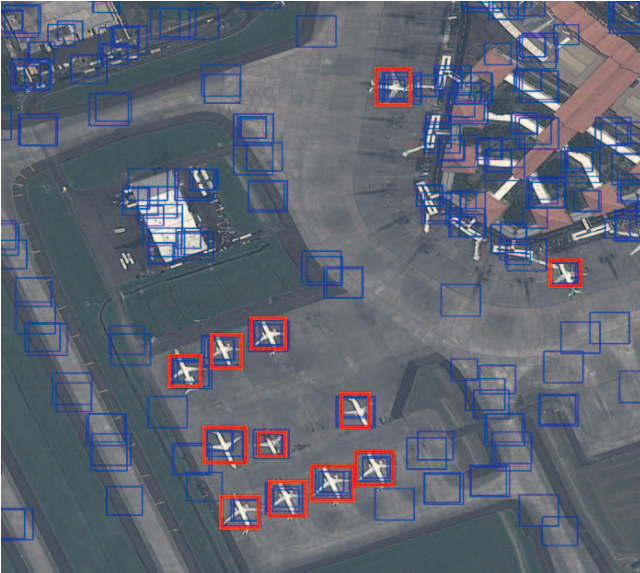
Fig. 7. A result of detection. Blue box: the proposal windows; Red box: the proposal windows after verification.
