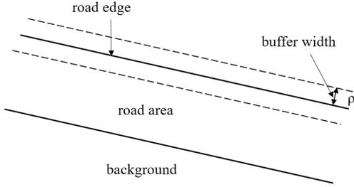
Fig. 2. The schematic diagram of edge-focused loss. The solid line represents the edge of the road, and between the two solid lines is the road area. We set the buffer width with  $\rho$ , and the area between the two dashed lines is the region where our loss focuses on learning.
