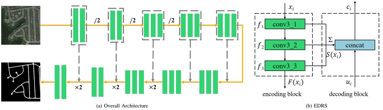
Fig. 1. The network structure of Richer U-Net. (a) Overall Architecture. /2 represents the pooling operation, and  $\times 2$  represents the upsampling operation. The area of gray dotted line stands for EDRS; (b) Enhanced Detail Recovery Structure (EDRS). Take the third level of convolution layers as an example, the structure includes an encoding block and a decoding block, and the output of the three convolutional layers is fused for the detail recovery in decoding block.
