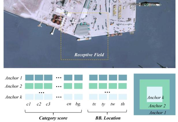
Fig. 4. An example of respective field and its multi-anchor boxes. For each anchor scale, the ground-truth label is arranged as two parts: category score and bounding box location coordinates. The final ground-truth label of the respective field can be formed by end-to-end connection of the label of each anchor scale.
