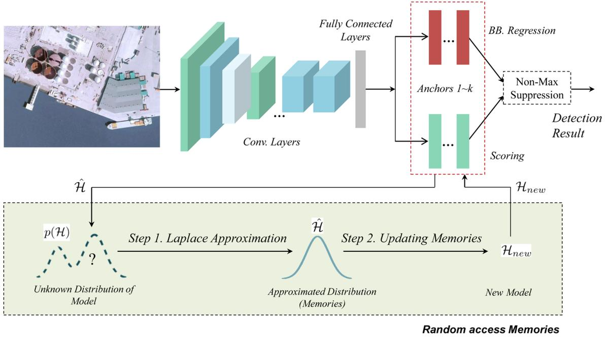
Fig. 3. A detailed Overview of our proposed new detection paradigm: backbone of the detector and random access memories. The RAM contains three steps: 1) Approximating the unknown distribution  $p(\mathcal{H})$  from  $\hat{\mathcal{H}}$  by Laplace Approximation, 2) updating the memories to get the new detection model  $\mathcal{H}_{new}$ .
