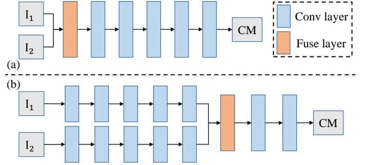
Fig. 9. Illustration of different neural networks architectures for merging the bi-temporal information. (a) Early fusion. (b) Late fusion.
