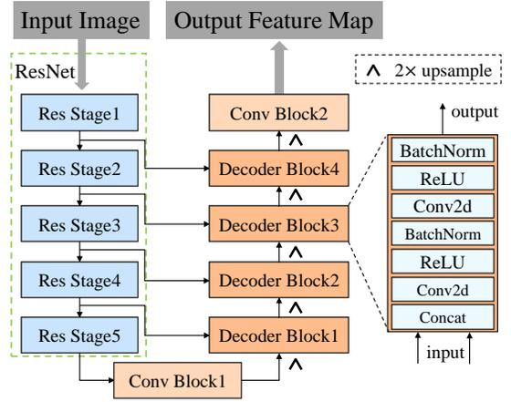
Fig. 10. Structure of the feature extractor.
