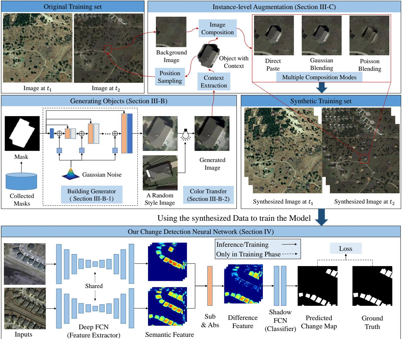
Fig. 2. Illustration of our proposed method. (Top) Procedure of synthesizing CD samples. (Bottom) Change detection model.
