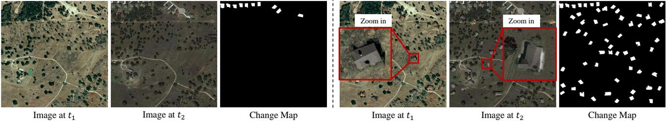
Fig. 1. An example of a CD sample in the LEVIR-CD dataset [6]. (Left) An original CD sample. (Right) The synthesized CD sample using our instance augmentation method.
