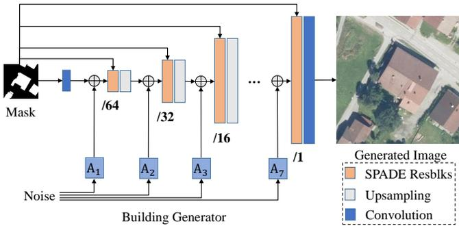
Fig. 4. Architecture of our building generator.
